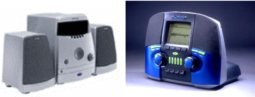
Figure 23: Two Web Radios: Two Internet appliances for browsing streaming audio are shown. On the left is the iRad 19 and to the right the Kerbango 20 . Each appliance bypasses the PC and accesses audio over the Internet directly.
