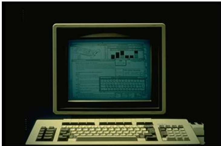
Figure 1: The Xerox Star 8010 Workstation. Introduced in 1981. This is the first commercial system to utilise a "windows, icon, menus, pointer" (WIMP), or "graphical user interface" (GUI).
