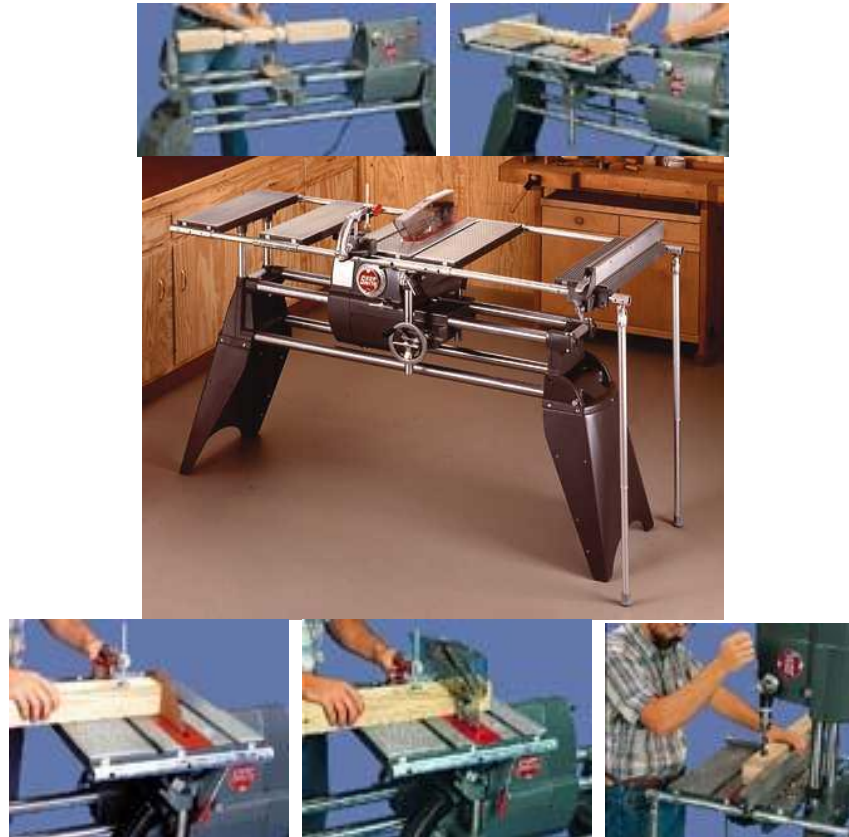
Figure 11: The Shopsmith: a 5-in-1 Powertool. The unit is shown along with each of its five different ways of being used.
